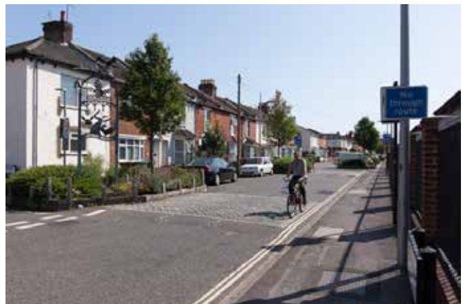
Figure 54 Signage, planting and a changes in surfacing indicates that the street is a Home Zone, a residential space designed to be safely shared by people, children and vehicles (Northam Home Zone)
